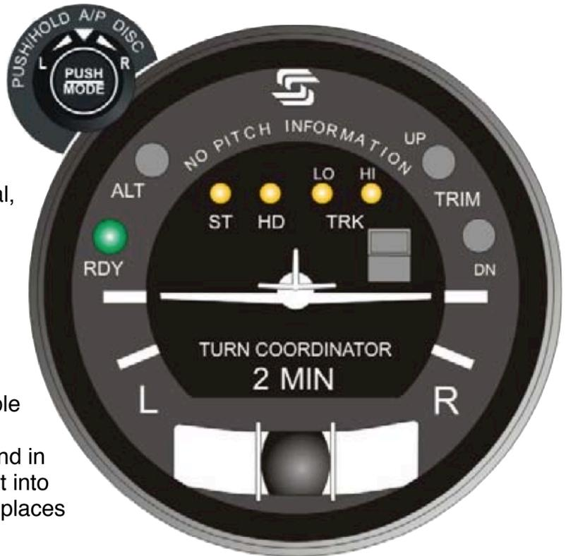
The TC component of the autopilot operates exactly as the instrument it replaces, complete with a red flag indicating that electrical power to the instrument has been lost. The TC powers up along with the battery master as usual.
